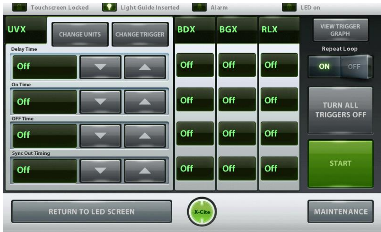
Figure 24 LED Trigger Screen (Touch Screen Controller)
