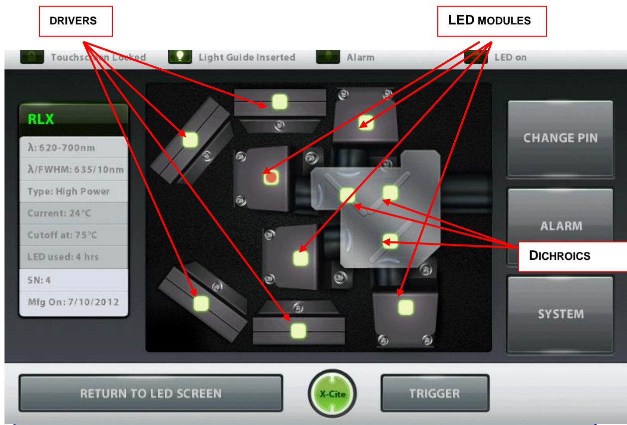
Figure 15 Maintenance Screen (GUI)
